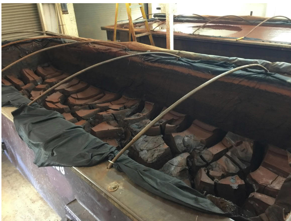
Figure 18: Chrome Treatment Train – Dewatering Beds
