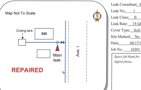
Leak Consultant: BC Leak No: 1 Leak Class: II Leak Rate: 15 GPM Cover Type: Soil Site Marked: No Date: 06/17/16
